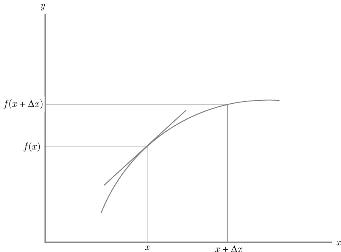
**Figure 2:** Determining slope of a nonlinear function at coordinates  $(x, f(x))$ .
